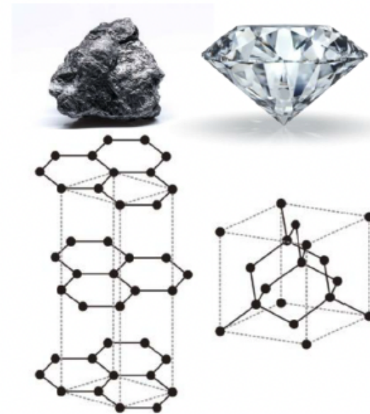
Figure 1: Graphite ( sp^2 ) and diamond ( sp^3 ) structure
