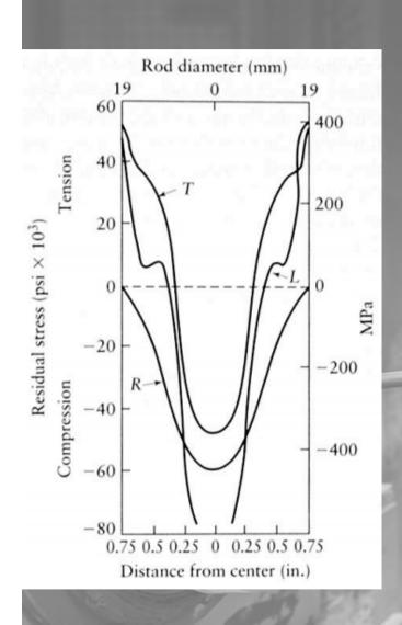
Because of the inhomogeneous deformation that the material undergoes, typically residual stresses occur in three directions:
